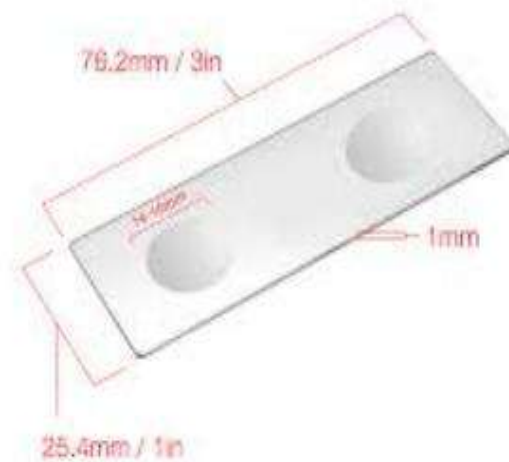
Figure 13.3: Dimensions of universal slide
