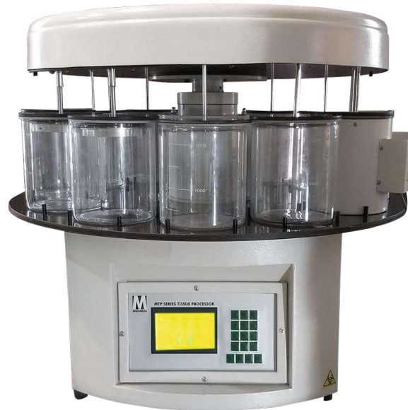
Figure 12. 1: Automated Tissue Processor
